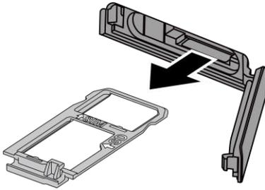
3. Put the tray onto a flat surface and place SIM or microSD cards into the tray with the gold contacts facing down as shown.
