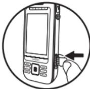
**Note:** With a memory card installed properly, the memory card icon appears at the top of the screen.
