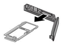
3. Put the tray onto a flat surface and place SIM or microSD cards into the tray with the gold contacts facing down as shown.
