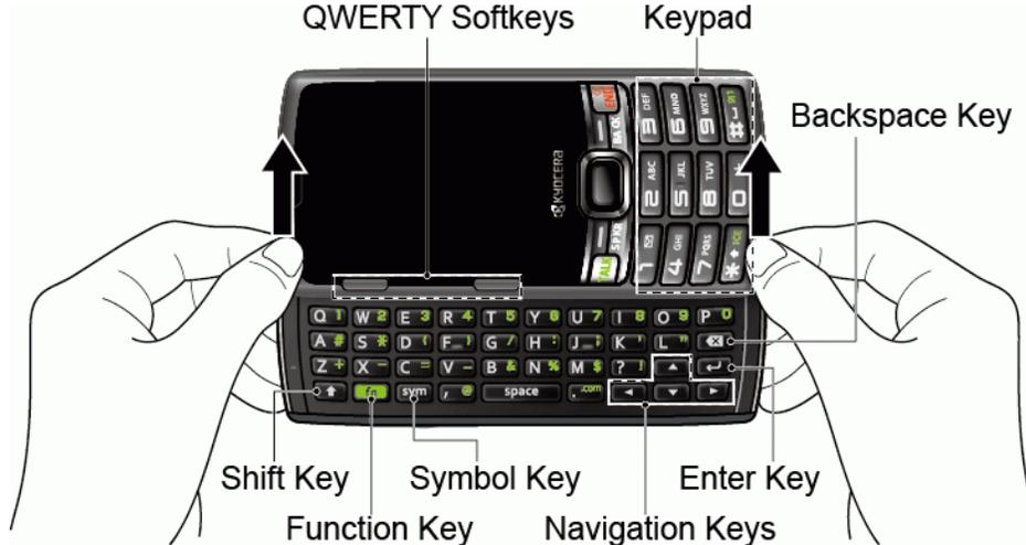
**Note:** When the slide-out keyboard is opened, the display stays in landscape mode and you can use the keypad on the front panel for entering numbers.
