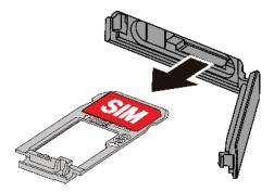
3. Put the tray onto a flat surface and place a microSD card into the tray with the gold contacts facing down as shown.
