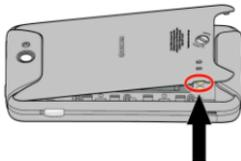
3. Insert the battery, contacts end first (①), and gently press the battery into place (②).
