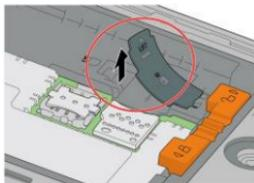
3. Insert the microSD card into the microSD card holder with the gold contacts facing down. Gently push the card in until it snaps into place.
