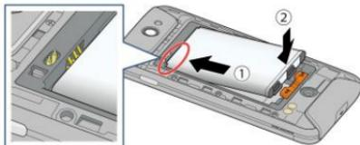
4. Slide the locking bar in the direction of the arrow to lock it.
