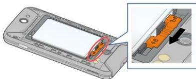
5. Replace the battery door, making sure all the tabs are secure and there are no gaps around the door.
