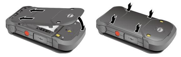
**Warning:** Make sure you press all around the edges of the battery cover to ensure your phone's waterproof seal is intact.
