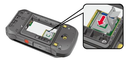
4. Carefully insert your new SIM card into the SIM card slot, with the gold contacts facing down and the cut off corner on the top left. Gently push the card in until it latches into place.
