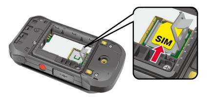
Note: Please be careful to not insert the SIM card into the SD card slot.
