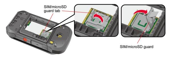
3. When a SIM card is already installed and you want to replace it, push the existing SIM card with your finger and then release the pressure. The card ejects itself. Slide it out from the slot.
